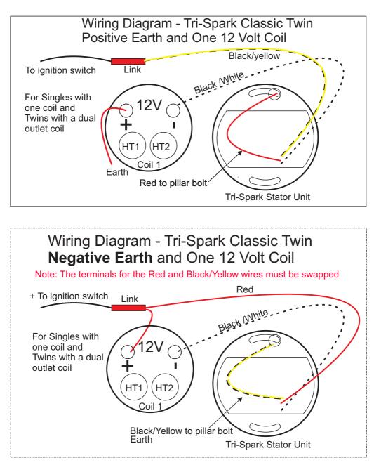
Note: **'To ignition switch'** means make connection with the wire intended for switching the ignition on/off at a convenient point. This is often a white/yellow wire that was originally connected to the negative side of the ignition coil(s) when running on points. Normally this connection is switched by the ignition and kill switches.
